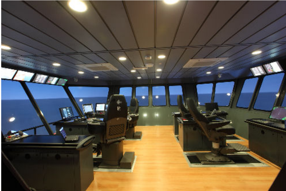
Figure 34 360 degree simulator 1: 360 degrees ship bridge simulator with traditional consoles. Functions: Dynamic positioning, propulsion control, visualisation, several different scenarios, anchor handling equipment, navigation etc.
