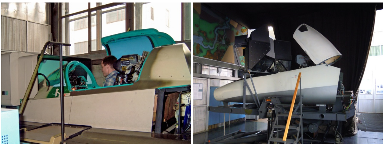
Figure 28 Ground-based simulators, with 60deg angle of view (left) and 120 deg angle of view (right)
