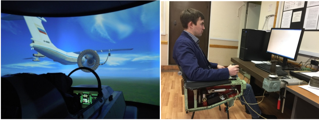
Figure 29 Flight Simulator with stereoscopy visual system – 180 deg angle of view (left) and two workstation for the manual control area research (right)
