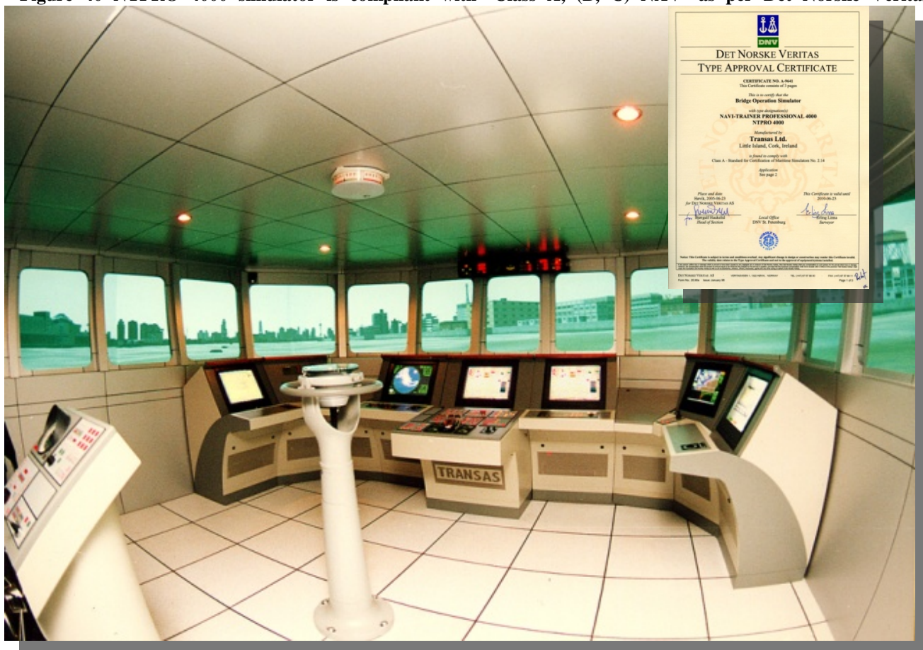
Figure 40 NTPRO 4000 simulator is compliant with ‘Class A, (B, C) NAV’ as per Det Norske Veritas
